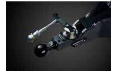
Steer by wire. Standard on the 7200 and 8400+ models. Optional on other models.
