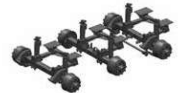
40 tons hydraulic suspended forced steered tridem
